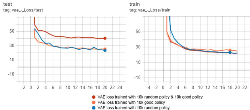
Figure 5.3: VAE test and train loss between VAEs trained with different datasets. The loss when using solely good or random policy rollouts was very similar. Combining both random and good policy data resulted in higher test loss, which might be due to the increased diversity of the data yielding a higher generalization error. Training a VAE with random policy rollouts was sufficient in representing different scenarios
