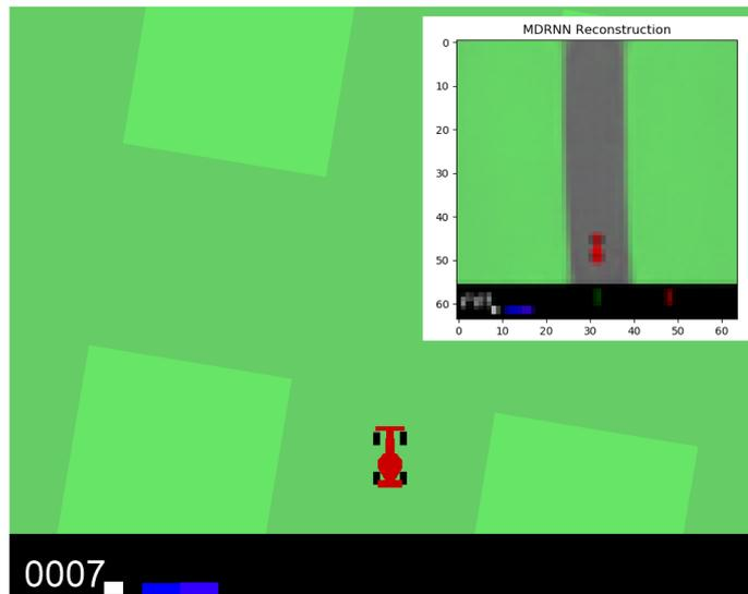
Figure 5.4: Comparison between model B MDRNN reconstruction against real frame. The model still believes the car is on the road, despite it being on grass. This is very likely due to bad driving samples being underrepresented when using good policy rollouts during MDRNN training
